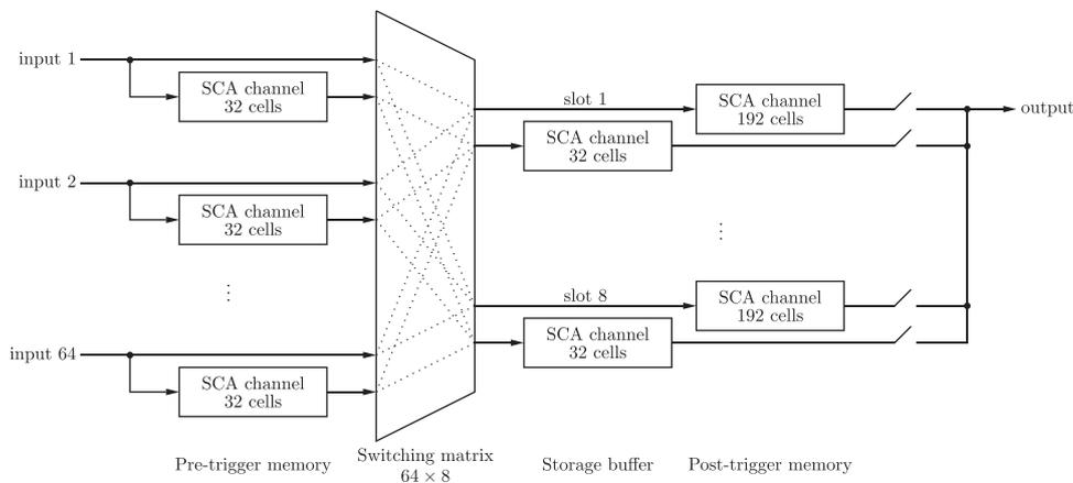
**Fig. 3.** Pipelined SCA architecture with separate channels for pre-trigger (left) and post-trigger (right) memory connected through a switching matrix. An additional channel in the right section acts as a storage buffer for the pre-trigger memory.
